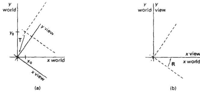
Figure 6-4 A viewing-coordinate frame is moved into coincidence with the world frame in two steps: (a) translate the viewing origin to the world origin, then (b) rotate to align the axes of the two systems.
